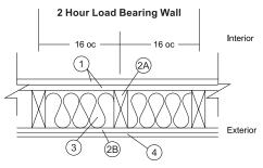
Max. Tested Load: 100% of Design Load
