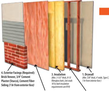
2B. FlamePRO Fire Retardant Treated Plywood (Min 15/32" thick • Optional color indicator for identification)
