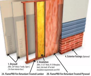
(Min 2x4, 16" o.c. • Optional color indicator for identification) (Min 15/32" thick • Optional color indicator for identification)
