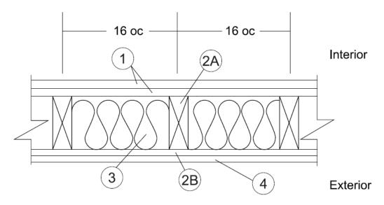
GYPSUM BOARD (Interior): Two-layers USG Firecode<sup>®</sup> C Core, complying with ASTM C1396, or equivalent, min. <sup>5</sup>/<sub>8</sub> in. thick, 4 feet wide applied vertically, fastened to framing. Face layer joints staggered with base layer and covered with paper tape and joint compound.
