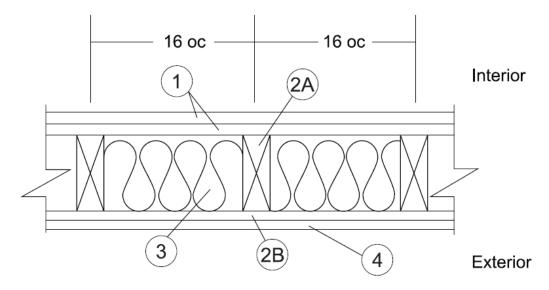
GYPSUM BOARD [Interior): Two layers Type C USG Firecode<sup>®</sup> C Core complying with ASTM C1396, min. <sup>5</sup>/<sub>8</sub> in. thick, 4 feet wide applied vertically, fastened to framing. Face layer joints staggered with base layer and covered with paper tape and joint compound.
